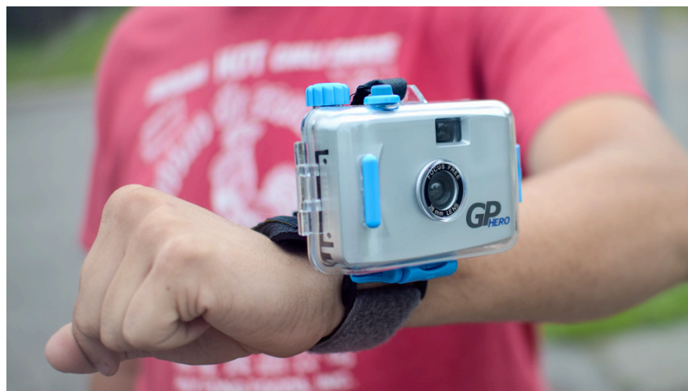
Figure 1: The original GoPro Hero camera was a wrist-worn, waterproof, 35mm photo camera developed by Nick Woodman in 2004. (© Philippe Bédard 2015)
